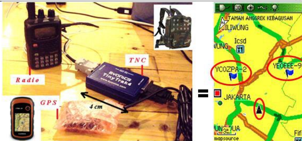
Fig. 6. APRS Schematic With Display [13]
